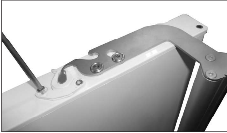
31. Go to the current door bottom and de-mount two screws from the door closer (use Torx 20 tool)
